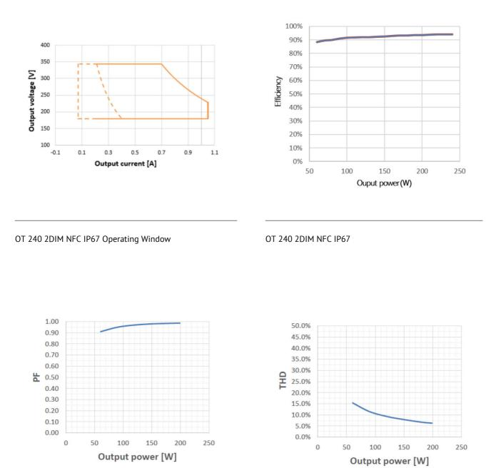
OT 240 2DIM NFC IP67 Typical Power Factor vs. Load
