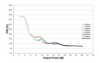
T FIT 30W CS Track Typical THD VS load
